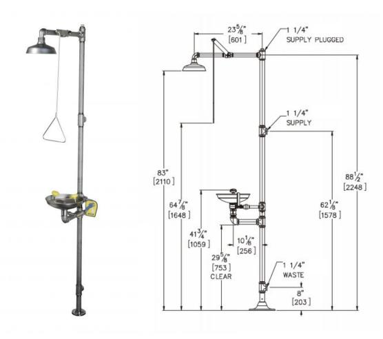
Model S2340-AS is our all stainless steel combined safety shower and eye wash with stainless steel head and yellow plastic spray heads. Complete with a 1" stainless steel stay open ball valve with stainless steel pull handle and activation lever for the shower and a 1/2" stainless steel stay open ball valve and stainless steel push handle for the eye wash.
